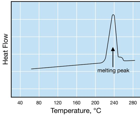
**Figure 4: DSC Analysis of a Part Injected in a Mold at 60°C (140°F)**
