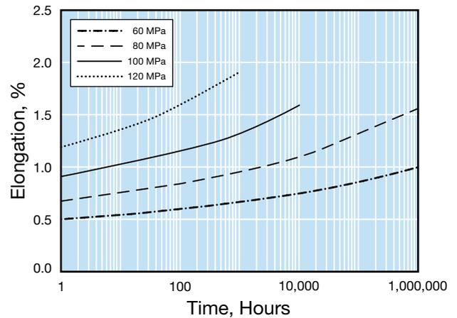
Figure 13: Tensile Creep of Ixef® 1022 with 2 mm Thickness at 120°C (248°F)
