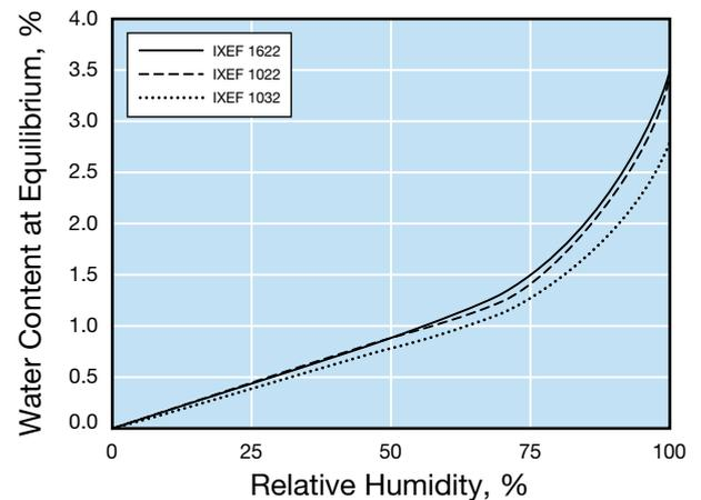
**Figure 21: Ixef® 1022 - FICK's Chart for Determining the State of Parts in Contact with Water or Water Vapor**
