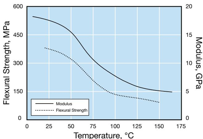
**Table 2: Flexural Properties of Ixef® PARA Grades (DAM) (ISO 178)**
