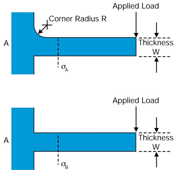
Figure 39: Stress Concentration Due to an Internal Corner
