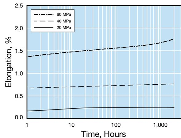
**Figure 14: Tensile Creep of Ixef® 1032 with 2 mm Thickness at 50°C (122°F)**
