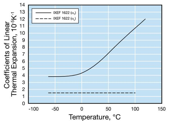
**Figure 19: Coefficients of Linear Thermal Expansion for Ixef® 2011**
