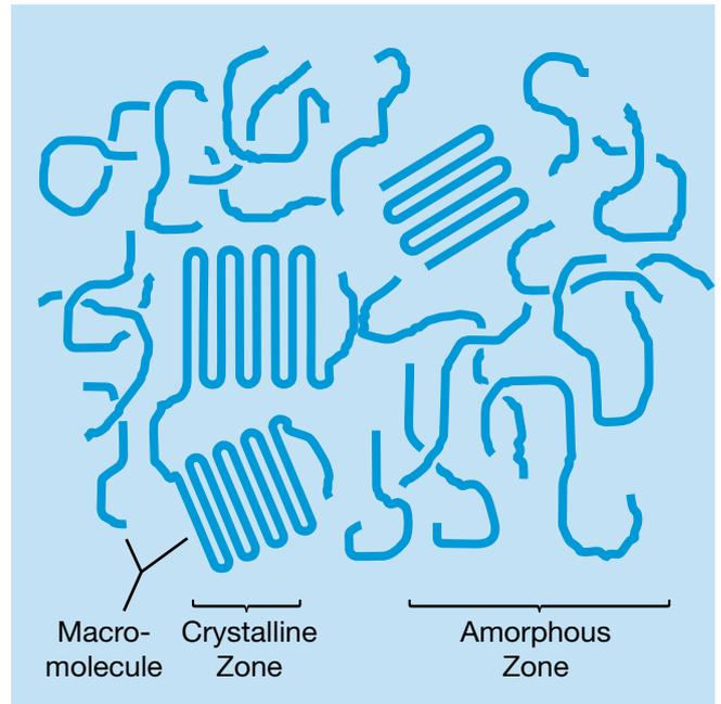
To develop a high crystallinity of Ixef® PARA compounds under normal injection molding conditions, it is essential to bring the temperature of the mold to between 120°C and 140°C (248°F and 284°F).
