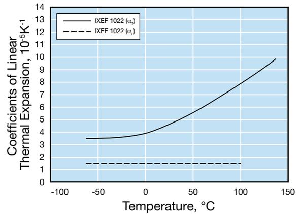
**Figure 18: Coefficients of Linear Thermal Expansion for Ixef® 1622**
