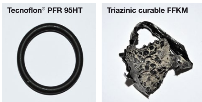
Effect of steam: 1 week @ 300^{\circ}\text{C}
