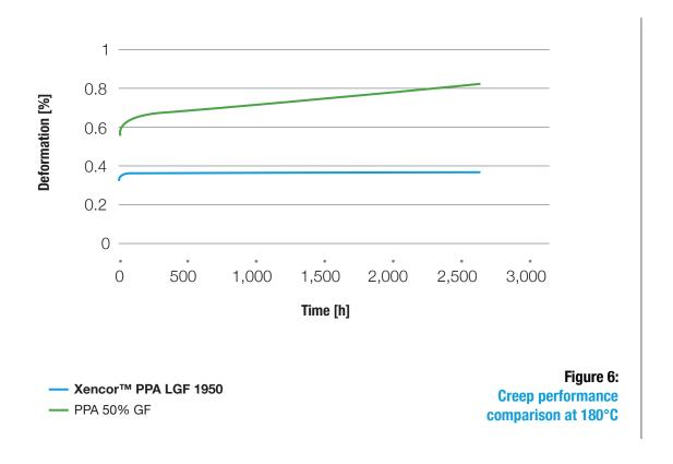
Typically, in creep, the fiber skeleton significantly limits the initial part deformation that occurs after load application as well as the increase in deformation over time. Long-term performance can exceed that of die-cast metals, such as Aluminum or Zinc, in particular at high temperatures.
