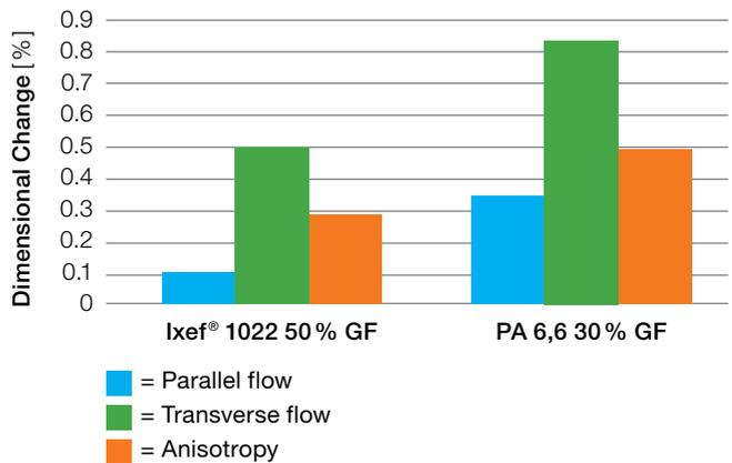
Test sample: 40 x 20 x 2 mm
