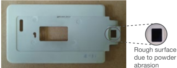
Figure 5: Specimen deflashed by blasting spray
