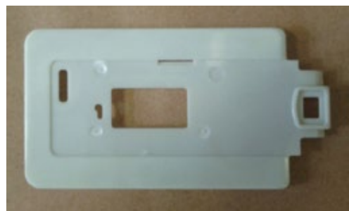
Figure 7: Specimen deflashed by cryogenic deflashing
