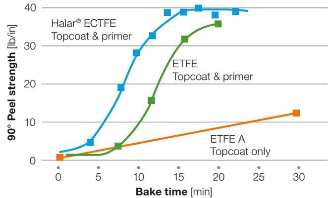
Adhesion test conducted using coating conditions recommended by the resin manufacturer. Halar® ECTFE is processed at 275 °C; ETFE at 315 °C. Primers are applied to develop maximum adhesion. The manufacturer of ETFE A recommends use of topcoat only.
