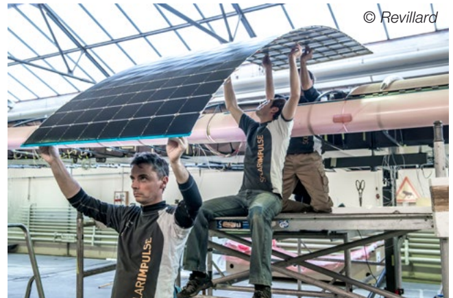
17 μ Halar® ECTFE film protect the over 17,000 solar cells of the Solar Impulse 2.
