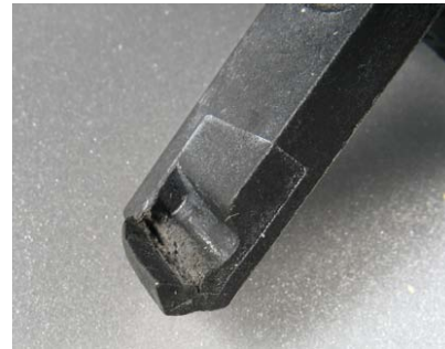
Figure 5: Unusual ductile failure of tab on thermostat housing
