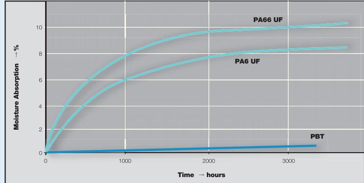
Figure 8. Dimensional stability of PA66 versus PBT
