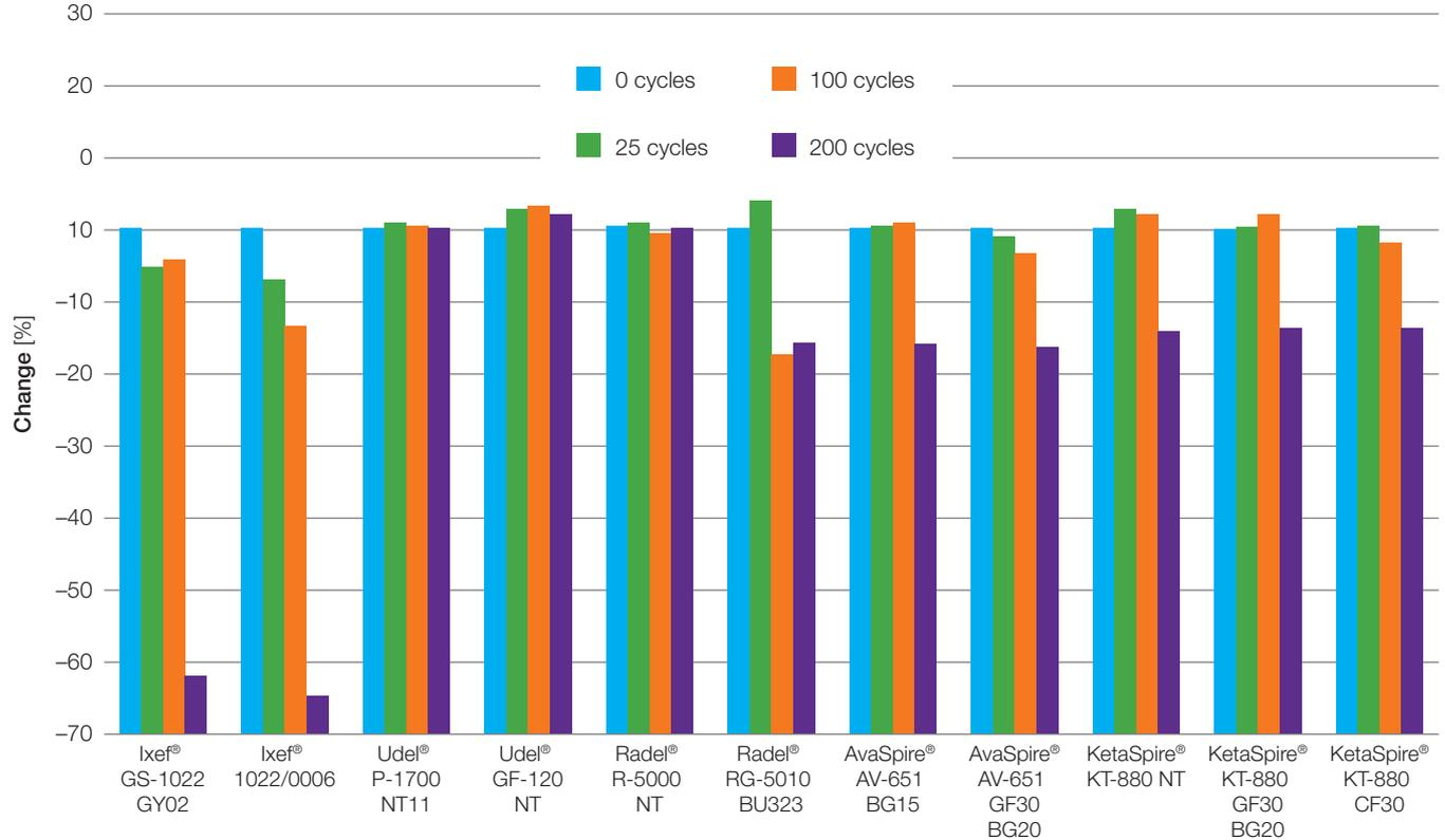
**Figure 13:** Weight Average Molecular Weight after Sterrad® 100NX® sterilization
