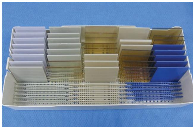
The load consisted of the Solvay test samples divided into two Sterrad® Aptimax® tray systems with mats. The samples were placed on edge and separated to maximize sterilant exposure around each sample (see Figure 1). The prepared trays were then double wrapped with polypropylene CSR wrap. The trays were placed on both
