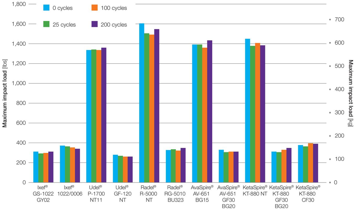
**Figure 8:** Instrumented impact energy after Sterrad® 100NX® sterilization
