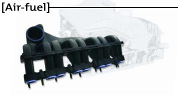
Replacing metal with Stanyl in air intake manifolds operating at higher temperatures and pressures, cuts production costs by up to 30% and reduces part weight by up to 50%.
