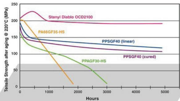
Our materials are able to fill very thin wall sections while maintaining the strength required to survive durability testing of the connection system and the individual contact isolation necessary for automotive environments. In addition, they exhibit strength in walls as thin as 0.1 millimeters and at weld lines.
