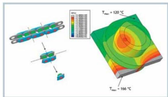
Figure 7; 3D dynamic thermal modelling reveals considerable local overheating at the chain to guide contact.
