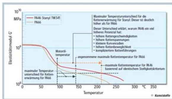
Figure 6; Modulus versus temperature of PA66 and PA46.
