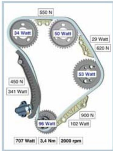
Figure 3; A timing chain layout with parasitic loss contributions due to sliding friction and chain articulation.
