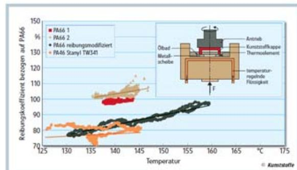
Figure 5; Graph comparing CoF of several materials versus temperature.
