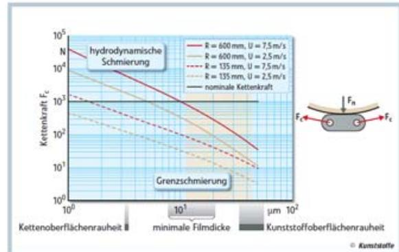
Figure 4; Lubrication regimes for chain-on-guide. Boundary lubrication occurs when the chain force is above the drawn curves.
