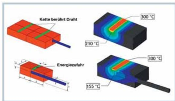
Figure 8; 3D dynamic thermal modelling reveals how the temperature profile in a plastic is distorted by introducing a thermocouple.
