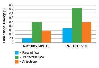
Test sample: 40 x 20 x 2 mm Test conditions: 750 bar, 280 °C Tooling: 120 °C, direct gating
