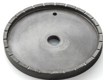
Figure 8.10: Thrustwasher test specimen with lubrication grooves
