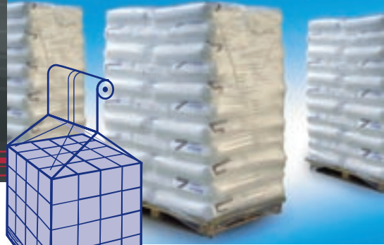
Fig. 8 Automation of pallet packaging. The film is pulled from the roll above the pallet.
